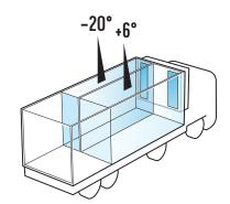
Special flexible unit with two different temperature zones.
